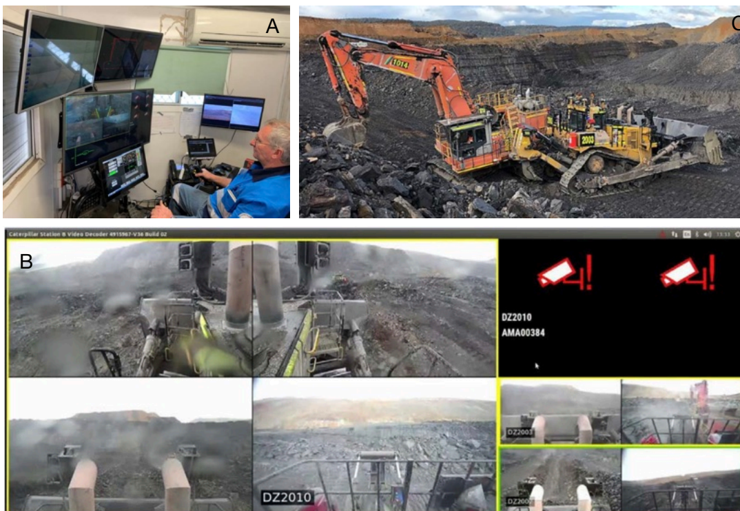
Figure 13: Remote operator station provided to the supervisor of three semi-autonomous dozers (A - top left); video images available (B - bottom) immediately prior to the collision between dozer 2003 and an excavator (C - top right).
