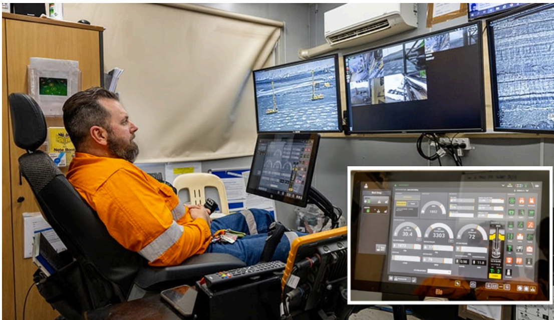
Figure 7: Replica drill cab workstation and interface for automated drill rig. (Westrac, 2022).
