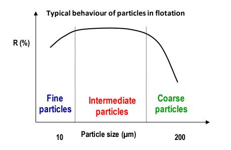
Fine and coarse particles have lower collection efficiency than the intermediate range
