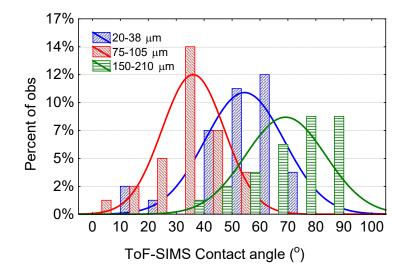
Fine and coarse particles need to be more hydrophobic than intermediate ones in order to float similarly for the same hydrodynamic conditions
