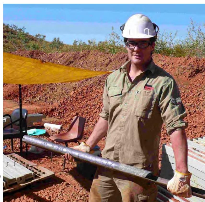
Figure 4.39 Merlin massive molybdenite breccia. 0.9m @46.4%Mo, 446g/tRe. Hole MDQ0264. Kirwin (2009)
