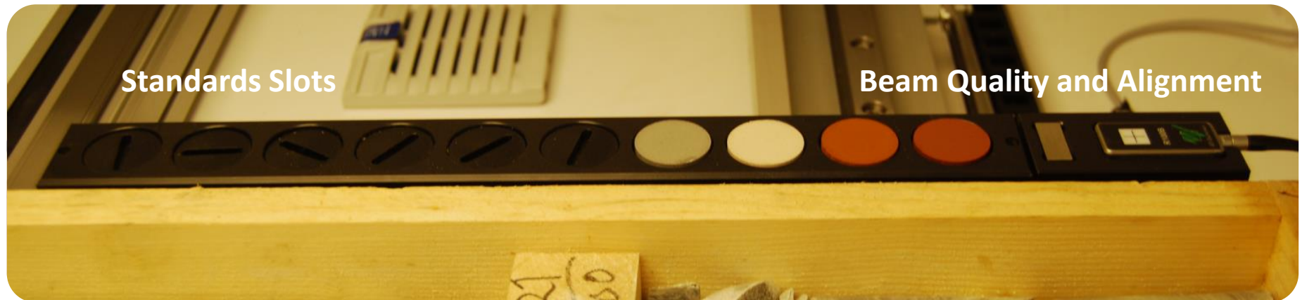
Calibration station integrated in Minalyzer CS for routine drift check and calibration.
