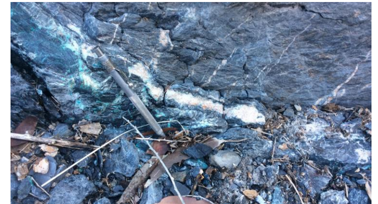
Shear failure and associated tensile veining, Cu mineralisation
