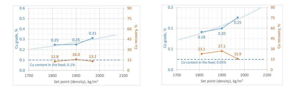
The valuable metals content in the sulfide concentrates was upgraded 2-3 times with up to 50% recovery rates, containing up to 0.40% wt. % Cu and 0.14 wt. % Co.
