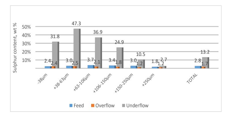
The decrease in sulfur content: ~40 wt. % on average, with the best results achieved for the +106-250  $\mu$ m particle size range – up to 65 wt. %.
