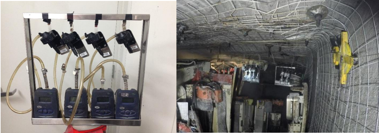
Figure 2- a) Respirable Cyclone Array on Frame b) Cyclone Array Mounted to Continuous Miner [7]
