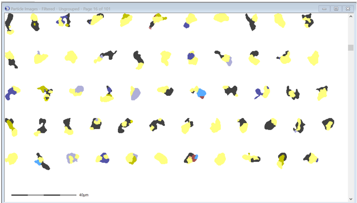
Figure 7- Images Particles containing >25% Silica Generated by the Minerals Liberation Analyser
